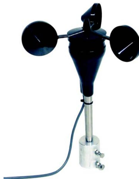
The **high performance MAX80+** anemometer has a **double resolution** compared to the MAX40+ anemometer and is standard supplied with MEASNET calibration certificate (example available on request). No power-supply needed.
